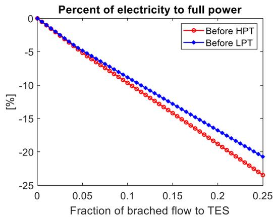
Fig. 4 The output change with branched flow into TES
