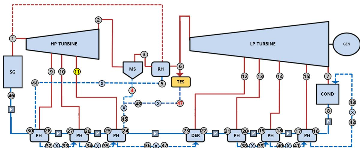
Fig. 3 Steam cycle layout of TES integrated NPP (Before LP turbine)
