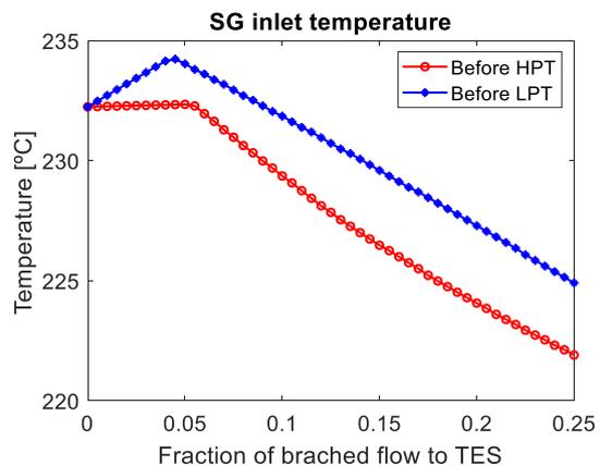
Fig. 7 The temperature change on steam generator inlet with branched flow into TES
