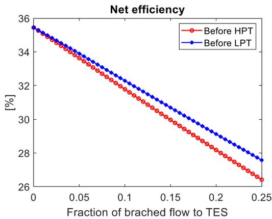
Fig. 5 The cycle efficiency with branched flow into TES
