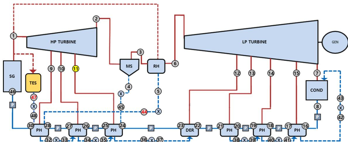
Fig. 2 Steam cycle layout of TES integrated NPP (Before HP turbine)
