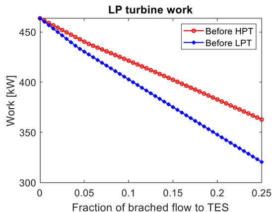
Fig. 9 The work of HP and LP turbine with branched flow into TES
