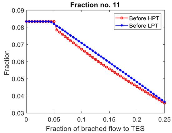
Fig. 6 The change of mass flow rate on HP turbine final extraction (no.11 on Fig. 2 and 3) with branched flow into TES
