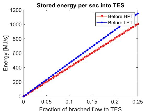
Fig. 8 The stored energy per second with branched flow into TES
