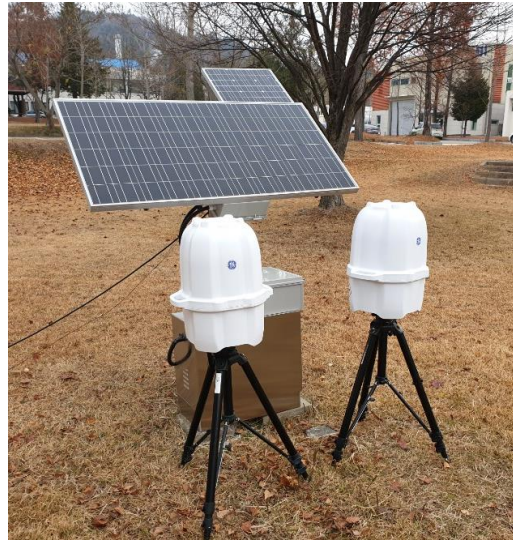
Fig. 3. Solar Panel based Radiation Monitoring System
