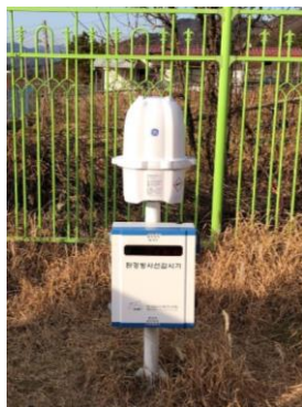
Fig. 1. Environmental Radiation Monitor deployed on site
