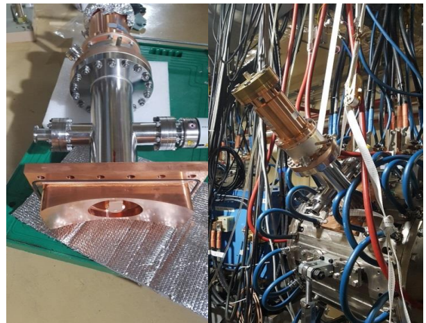
Fig. 3. Installed MEBT RF Coupler
