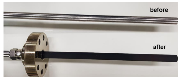
Fig. 2. Commercial steam generator tube (Alloy 690TT) used in this study (a) before and (b) after the experiment.
