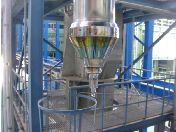
Fig. 3. New designed capsule out-pile tested for 23 cycles (690 days)
