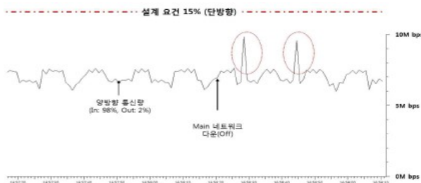
Fig. 4. Network traffic in Failover
