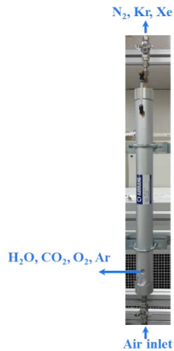
Fig. 5. Gas separation by the hollow-fiber membrane module.
