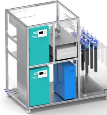
Fig. 7. Compact size of continuous H 2 O and CO 2 sequestered Kr-85/Xe isotopes sampling system.
