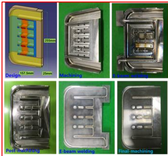
Fig. 3. Schematic diagram of the manufacturing process of the small mock-up of BZ-SW (Part-B)
