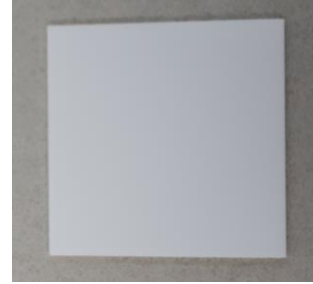
Fig. 1. Photo of a Al_2O_3 sheet (25 mm x 25 mm, thickness: 1.0 mm, Goodfellow).
