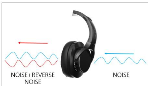
Fig. 1. Noise canceling principle
