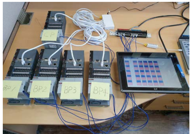
Fig 4. Prototype of integrity monitoring system for RPS using the blockchain
