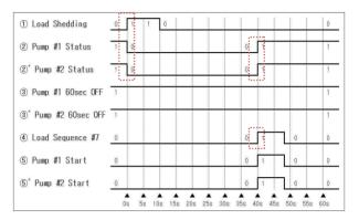
Fig. 4. Timing chart for the ESWP control signal in case of the LOOP during two ESWPs are running simultaneously in the train
