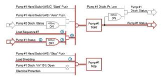
Fig. 1. The control logic for the ESWP
