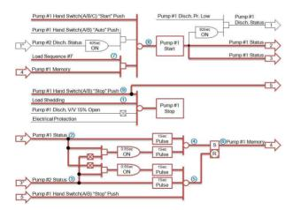
Fig. 6. The improved control logic for the ESWP
