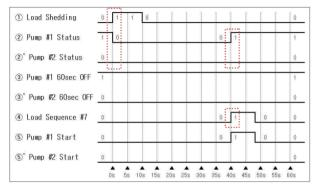
Fig. 2. Timing chart for the ESWP control signal in case of the LOOP during only one ESWP is running in the train
