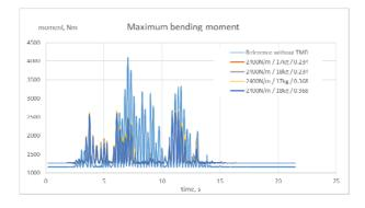
Fig. 4. Maximum bending moment in the entire piping system
