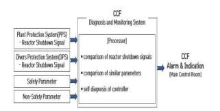
Fig. 1. The concept diagram for CCF diagnosis and monitoring system.
