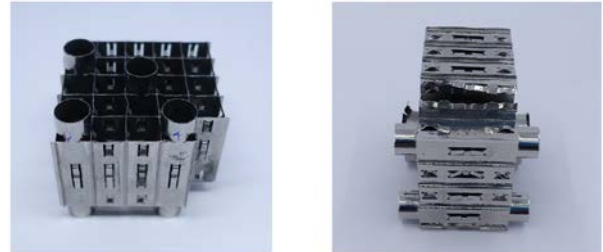
Fig. 4. Specimen after 4 hours of dry electropolishing (left) and after 4 additional hours (right)
