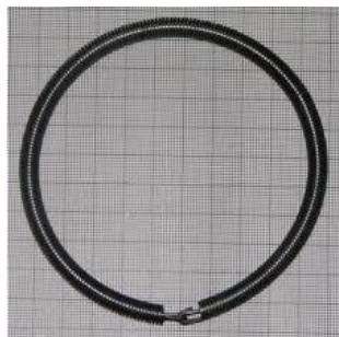
Fig. 1 CANDU fuel channel and spacer
