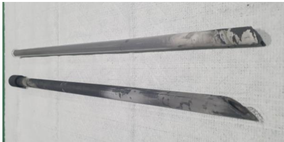
Fig. 2. Y_2O_3 coated quartz mold (above molds) and graphite mold (below molds) after casting
