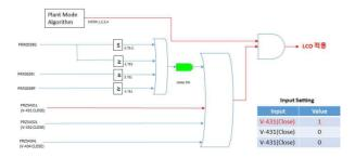
Fig. 4. The example of a logic diagram of the entry of LCO
