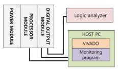
Fig. 2. Three elements of the NQ-D23QC's normal access
