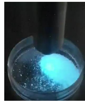
Fig. 8. Image of ZnWO_4 (650 rpm planetary ball milling for 5h) under 50 kV p X-ray tube
