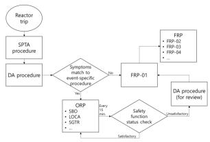
Fig. 1 General structure of a CE-based EOP system [4]
