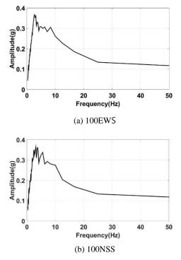
Fig 2. Spectra of horizontal seismic inputs.
