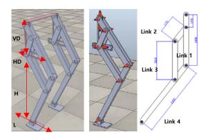
Fig. 2. 2DOFs pantograph leg mechanism.
