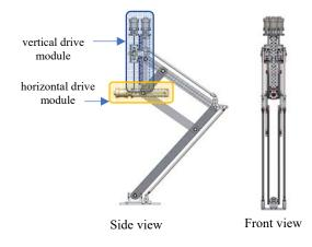
Fig. 4. The proposed pantograph leg design.
