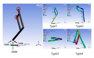
Fig. 3. A static FEM analysis model and results for 4 support conditions.
