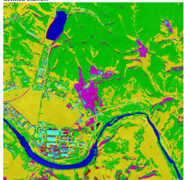
Fig. 5. Reclassification result where water classes (blue) was assigned from the misclassified objects considering MNDWI over 0.4.
