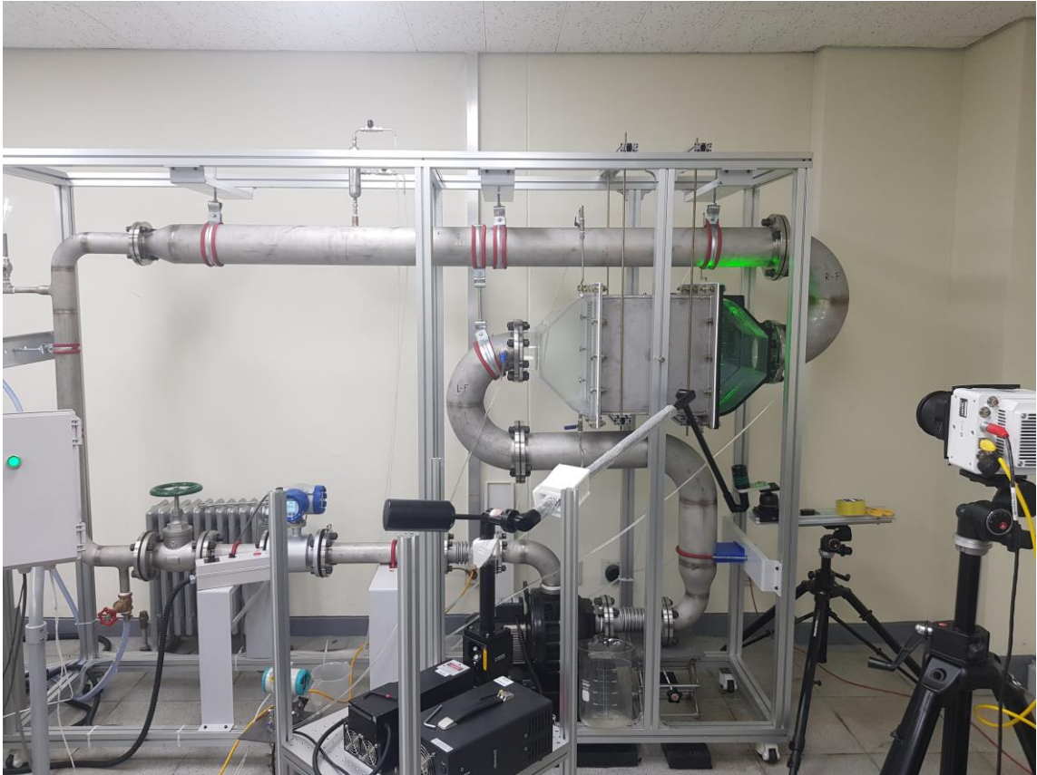
<Experimental loop and PIV configuration>
