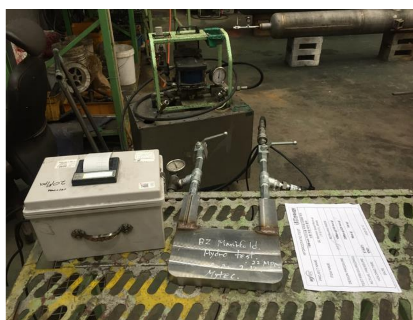
Water pressure test for mock-up of BZ-SW small mock-up
