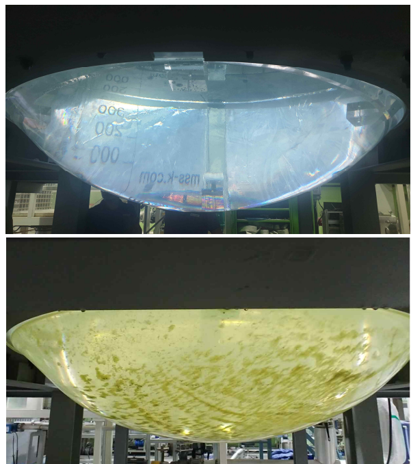
Figure 3. DTV-A01 Test Result - Lower Hemisphere Area of the Simulated Reactor Vessel
