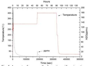
Fig. 5. Amounts of vapor on the desorption with various time (Red line : temperature, dashed line : ppmv)
