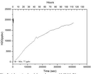
Fig. 3. Adsorption breakthrough curve : 10 SLM, 20 ppmv
