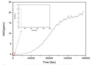
Fig. 4. Adsorption breakthrough curve : 2 SLM, 20 ppmv
