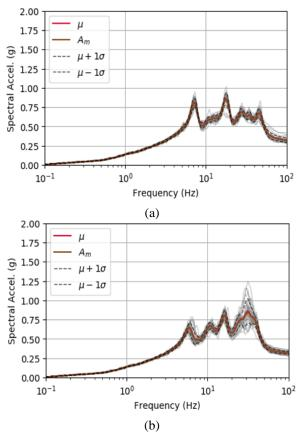
Fig. 4. Floor response spectrum of (a) uncracked and (b) cracked model.
