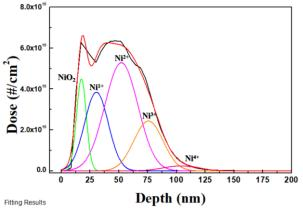
Fig. 3. D-SIMS data and fitting results of the Ni ion beam.
