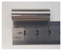
Fig. 2. The cathode for MEVVA ion source
