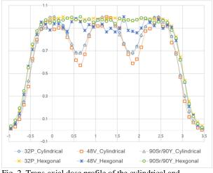
Fig. 2. Trans-axial dose profile of the cylindrical and hexagonal models (0.5 mm wall thickness), for various radioactive sources at a depth of 2.5 mm.
