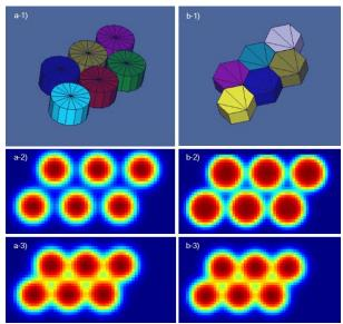
Fig. 3. In MCNP6 simulations, a-1) and b-1) show the 3D shapes of six applicators. a-2) and a-3) show the dose distribution of cylindrical models using <sup>32</sup>P, for wall thicknesses of 2 mm and 0.5 mm, respectively. b-2) and b-3) show the dose distribution of hexagonal models using <sup>32</sup>P, for wall thicknesses of 2 mm and 0.5 mm, respectively.
