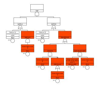
Fig. 2. ITE-based fault tree modeling of two HFEs and their dependency
