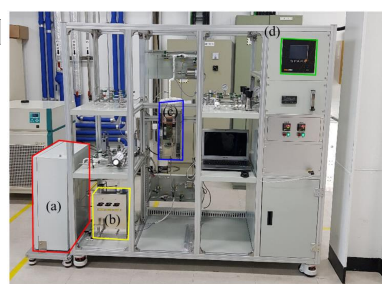
Figure 5 Layout of the AMSB apparatus: (a) dryer, (b) vapor generator, (c) test section with a furnace and (d) vapor analyzer
