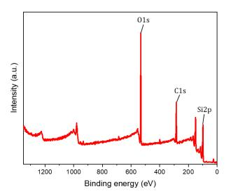
Fig. 3. XPS element survey of  $SiO_x$  nanoparticles synthesized at 7.5 V.
