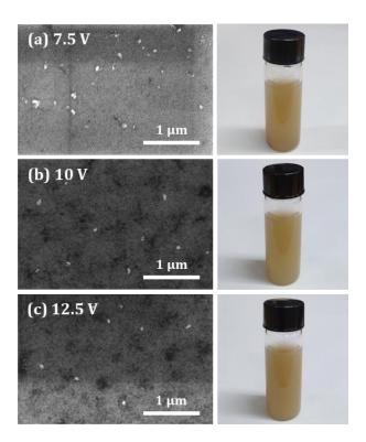
Fig. 2. FESEM images and digital photographs of  $SiO_x$  nanoparticles synthesized at each anodization voltage; (a) 7.5, (b) 10, and (c) 12.5 V.
