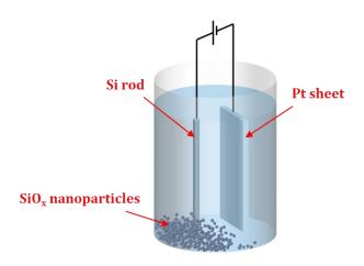
Fig. 1. Schematic view of anodization system.
