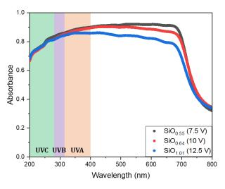
Fig. 5. Photon absorbance of  $SiO_{0.55}$ ,  $SiO_{0.64}$ , and  $SiO_{1.01}$  nanoparticles.
