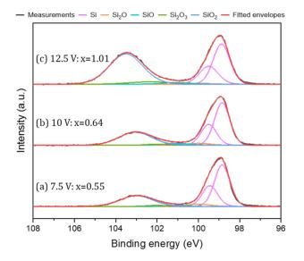
Fig. 4. XPS Si 2p spectra of SiO<sub>x</sub> nanoparticles synthesized at each anodization voltage and calculated x-values after peak deconvolution; (a) 7.5, (b) 10, and (c) 12.5 V.
