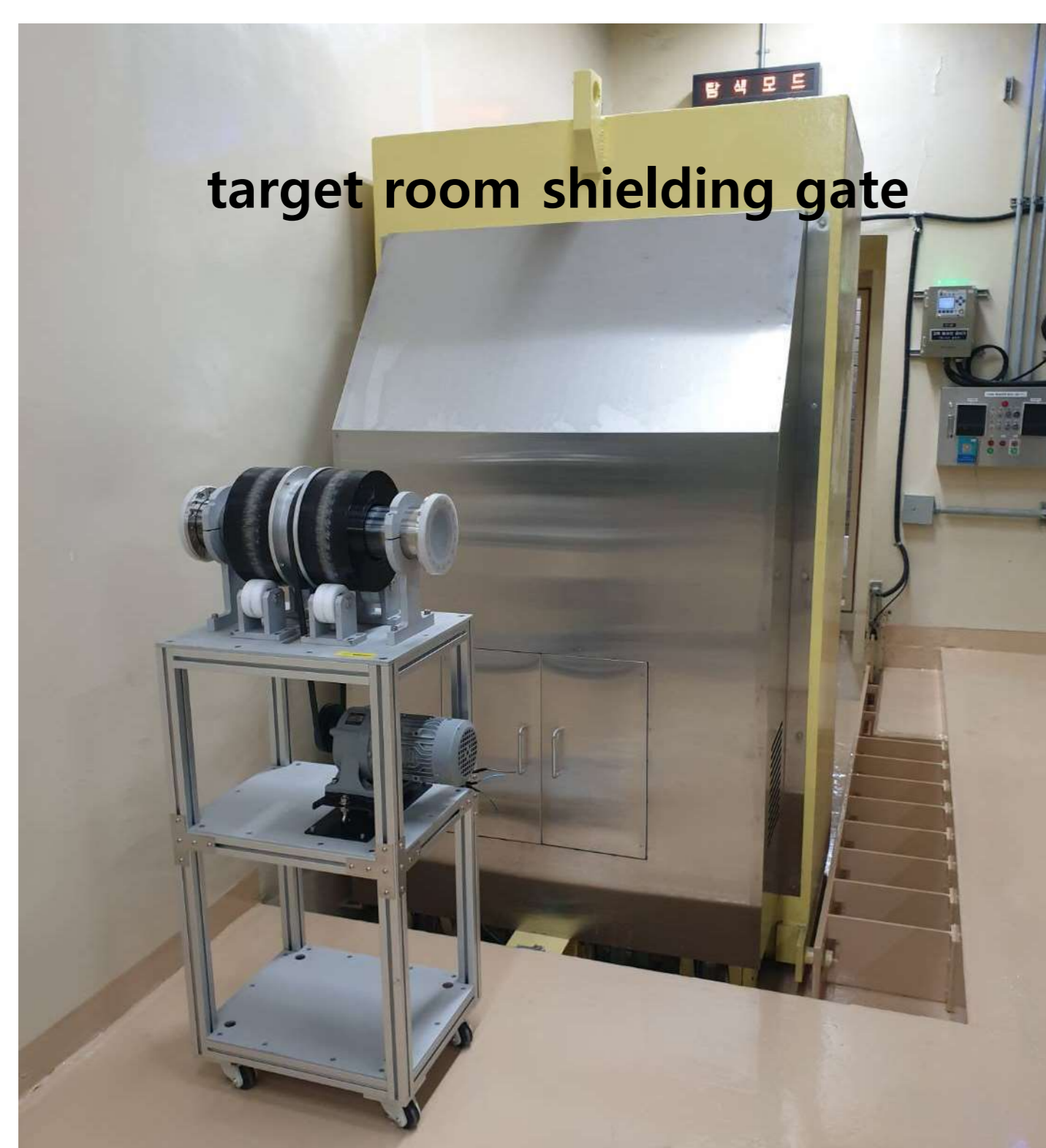
Wobbler waiting installation
