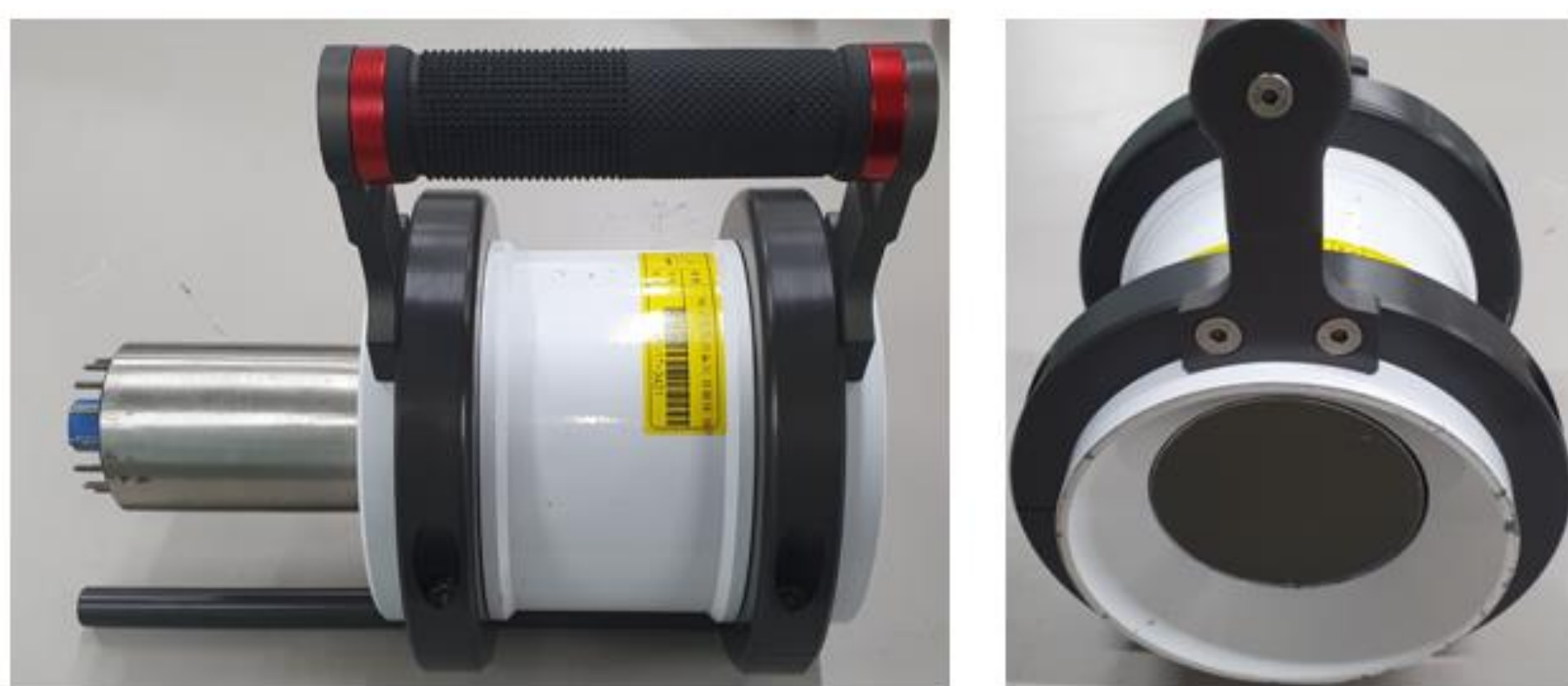
Figure.1 45° collimator for 3inch NaI(Tl) detector
