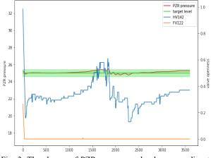
Fig. 3. The change of PZR pressure and valves according to the timestep in the last episode.
