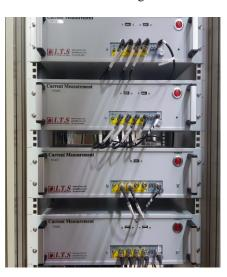
Fig. 3. The wire scanner control units installed in KOMAC beamlines.
