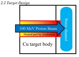
Figure 2. Simplified diagram of the target with cooling water channel.
