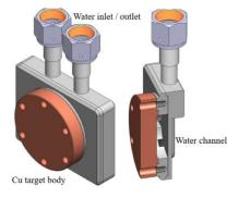
Figure 5. Drawings of Cu target body.
