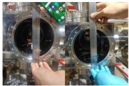
Figure 6. Picture of target installation inside a beam line chamber, when the target is in use (left) and removed (right)
