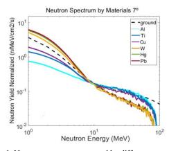
Figure 1. Neutron spectrum generated by different materials compared with atmospheric neutron at ground level.
