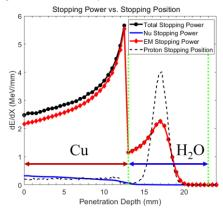
Figure 3. Stopping power characteristics of a 100 MeV proton beam impinging on the target assembly consisting of a 13mm-thick Cu target body and 10-mm-thick cooling channel
