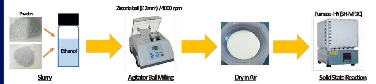
• Fabrication of Transparent ZnWO<sub>4</sub> Thin Film
