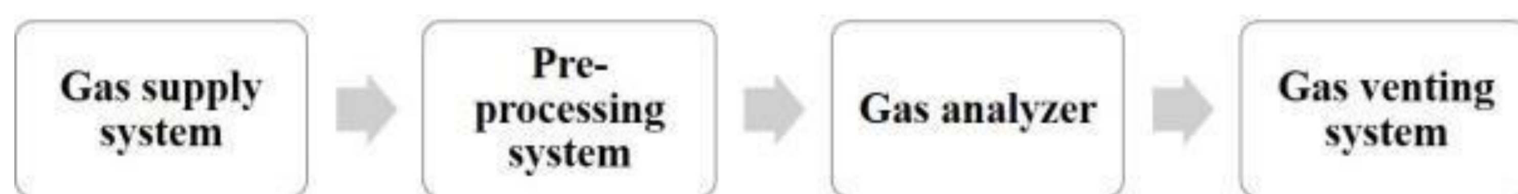
Process of gas analysis system of SPARC test facility
