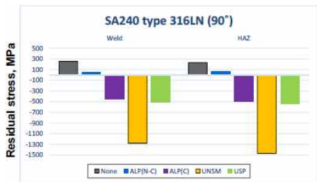
Figure 5-2. XRD Measurement Results (Avg. Value) Comparison Table (Type 316LN, 90° direction)
