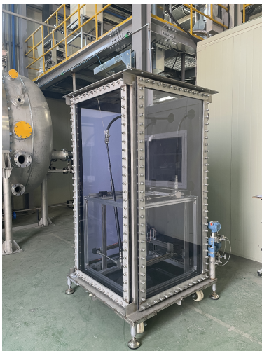
Figure 1. visible water tank
