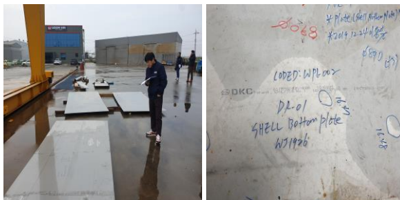
Fig. 2. Acceptance and visual inspection
