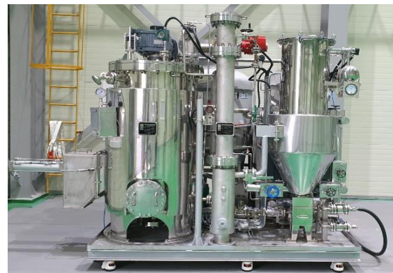
Fig. 7. Drying facility of centrifugal thin-film type
