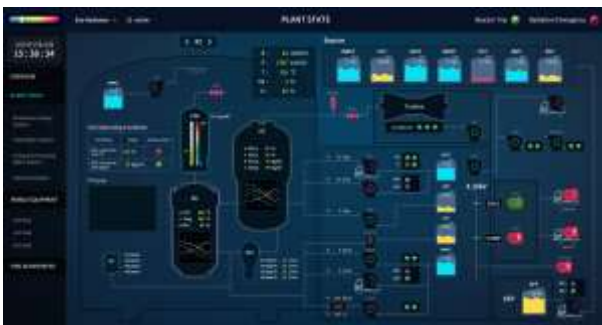
Fig. 3 Snapshot of plant status of the MOAS. Every cooling assets are depicted with important plant parameters and mobile emergency facilities.
