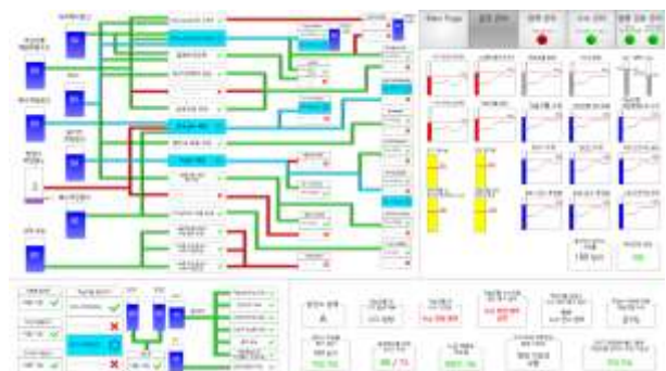
Fig. 10 Snapshot of lower-level abstraction of the EID. Possible cooling paths, state of important parameters and supportive information are shown along with selected metric (temperature, level, radioactivity, pressure)
