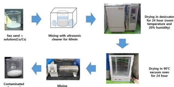
Fig. 1. Procedure for preparing contaminated sea sand
