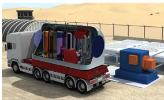
Fig. 2. S-CO 2 coupled distributed power system concept diagram (KAIST-MMR) [2]
