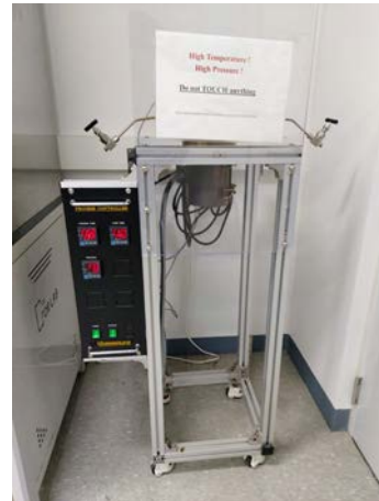
Fig. 1. Static autoclave corrosion test apparatus.
