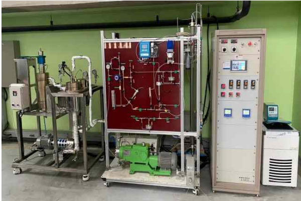
Fig. 2. Flow accelerated corrosion test facility.
