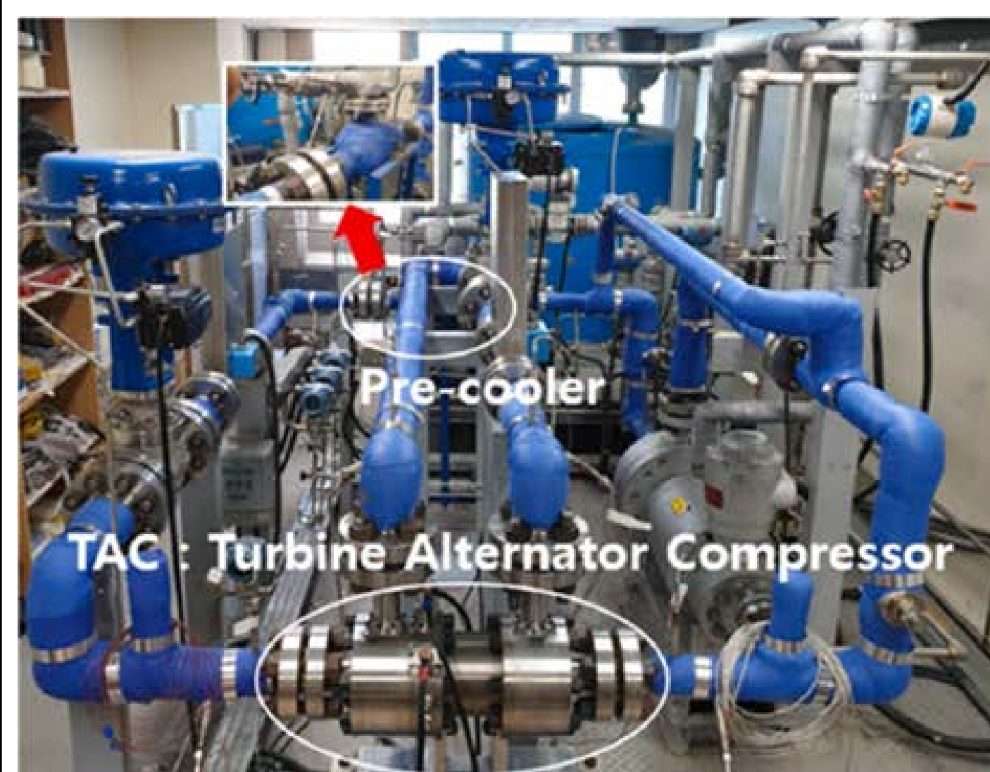
▲ Compressor performance test loop in KAIST and schematic diagram
