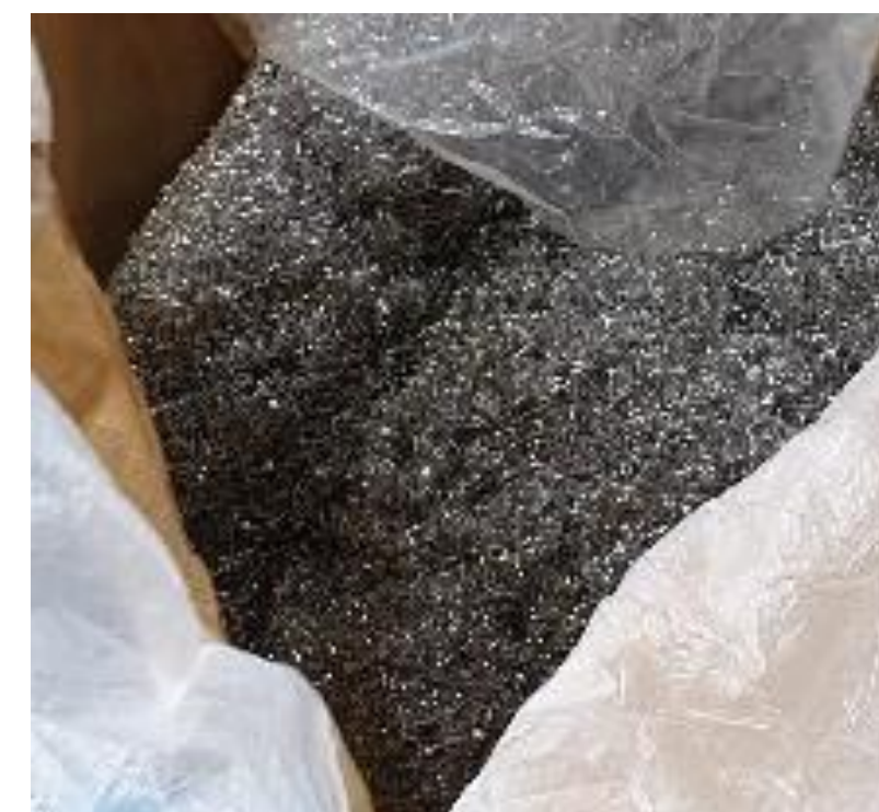
Picture of aluminum chip and aluminum cladding which were generated during manufacturing nuclear fuel.
