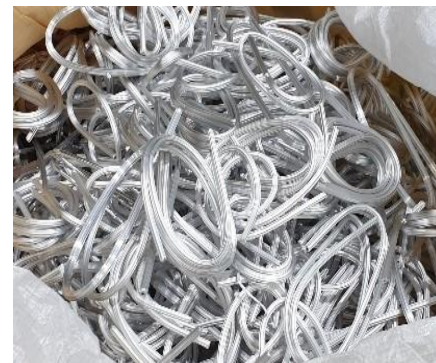
Picture of aluminum chip and aluminum cladding which were generated during manufacturing nuclear fuel.
