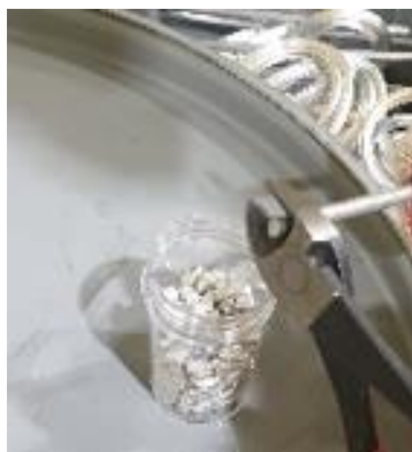
Picture of selecting and weighting of aluminum chip and cladding sample
