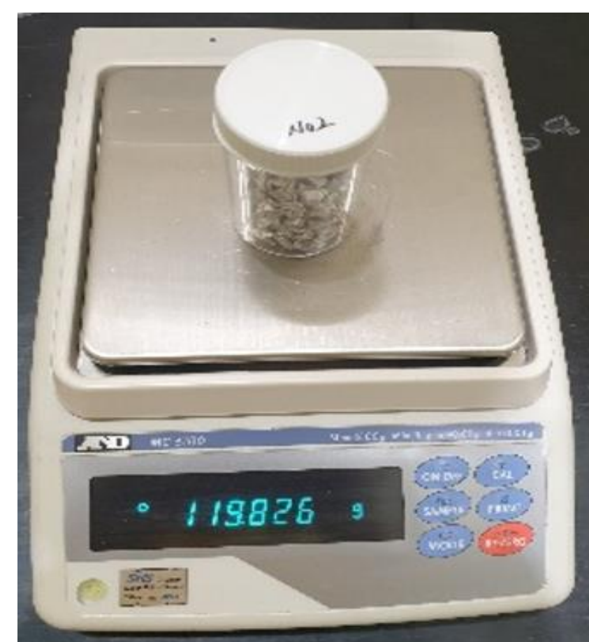
Picture of selecting and weighting of aluminum chip and cladding sample
