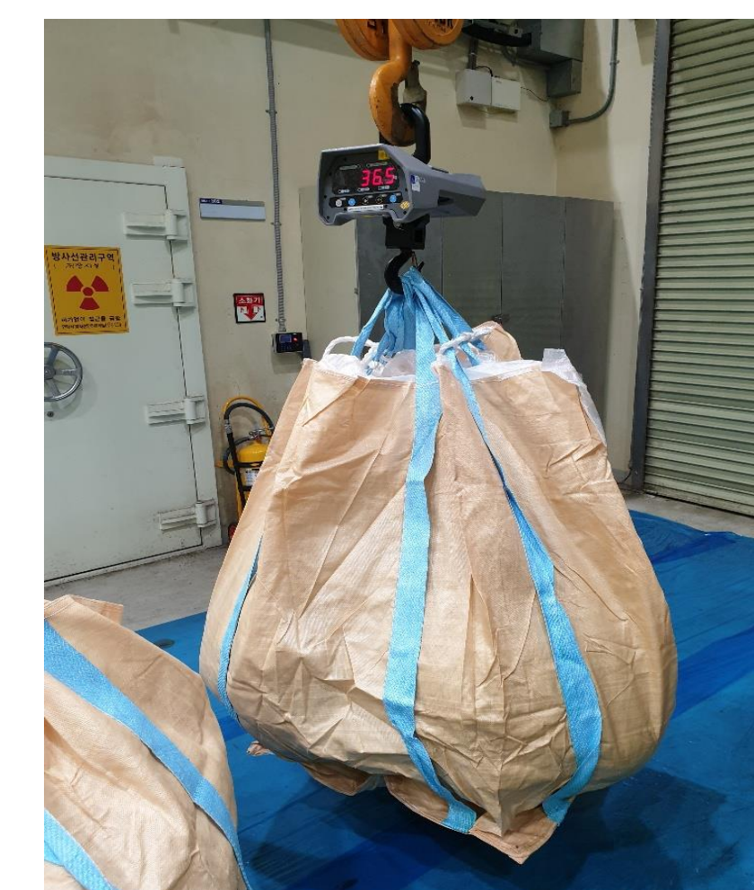
Picture of weight measurement using calibrated weighing machine.
