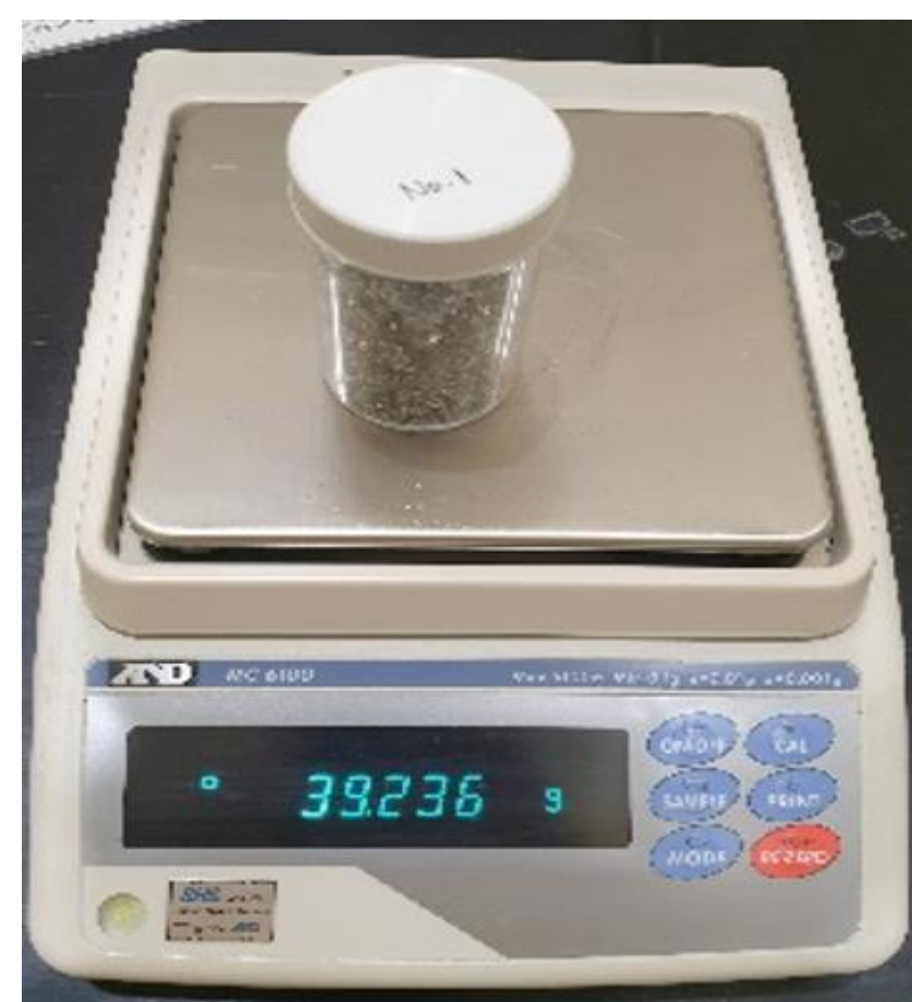
Picture of selecting and weighting of aluminum chip and cladding sample
